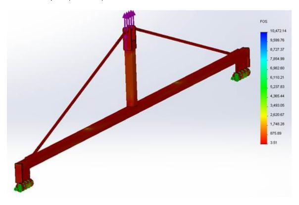
I don't see any structural issues with the above lifting assemblies as the safety factors are all well above 2. I'm currently working on drawing 95-1109 and should have results for you tomorrow. Feel free to call me with any questions/concerns.
